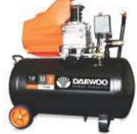
Compresor Daewoo DAC50D (29022) •2 HP •Cap. 50 Lts. •Caudal 195 L/min. •220 V •2850 rpm
